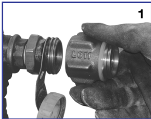
Screw LG11 to fill point fitting.
