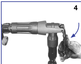
After refuelling disengage lever, prepare for disconnection.
