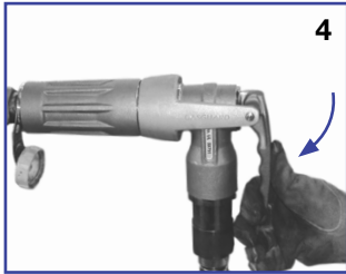
After refuelling disengage lever, prepare for disconnection.
